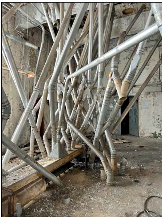
Spouts and wheat feeders on the 6 th floor. (Photo on right: Ben Halpern).
