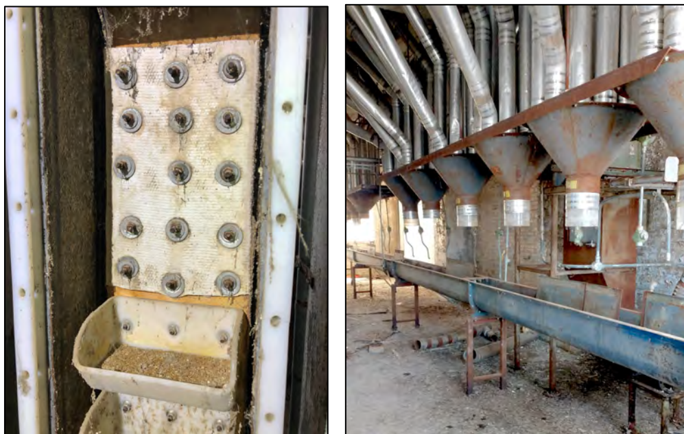
Spliced elevator belt, with product cups (left). Smutter’s wet wheat mixer (right).
