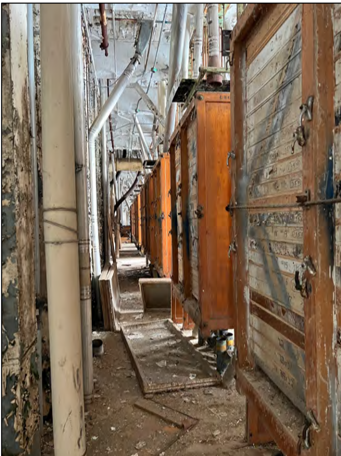
Eighth floor wooden sifters, suspended from the ceiling. Note drawer-like screens, and diagonal reference lines painted by staff to replace screens in proper position. (Photo on left: Chris Richmond)
