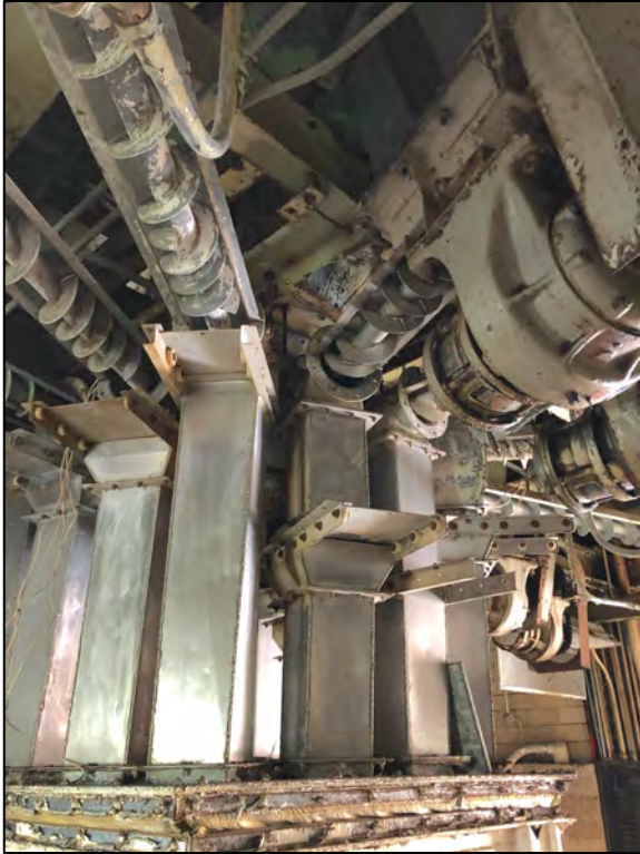
Product augers on the 5 th floor (above), ingredient shoots (7 th floor), and view of 8 th floor (right).
