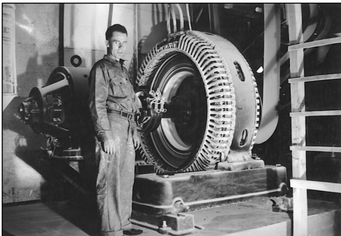
Motor used to drive mill stands (left) and bakers in the test kitchen (right), circa 1930s.
