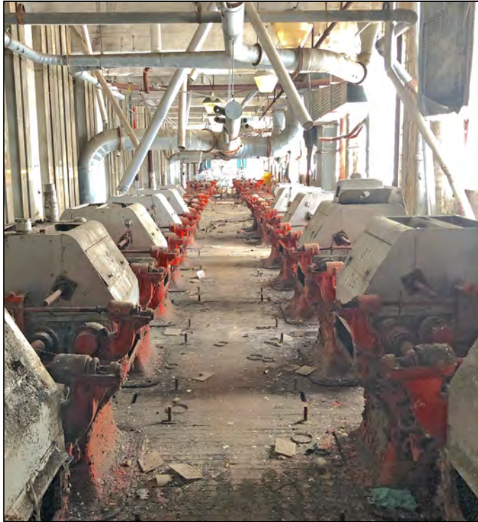
Fourth floor mill stands or “bolt stands”. On right, two large rollers and a grain separator inside the stands.
